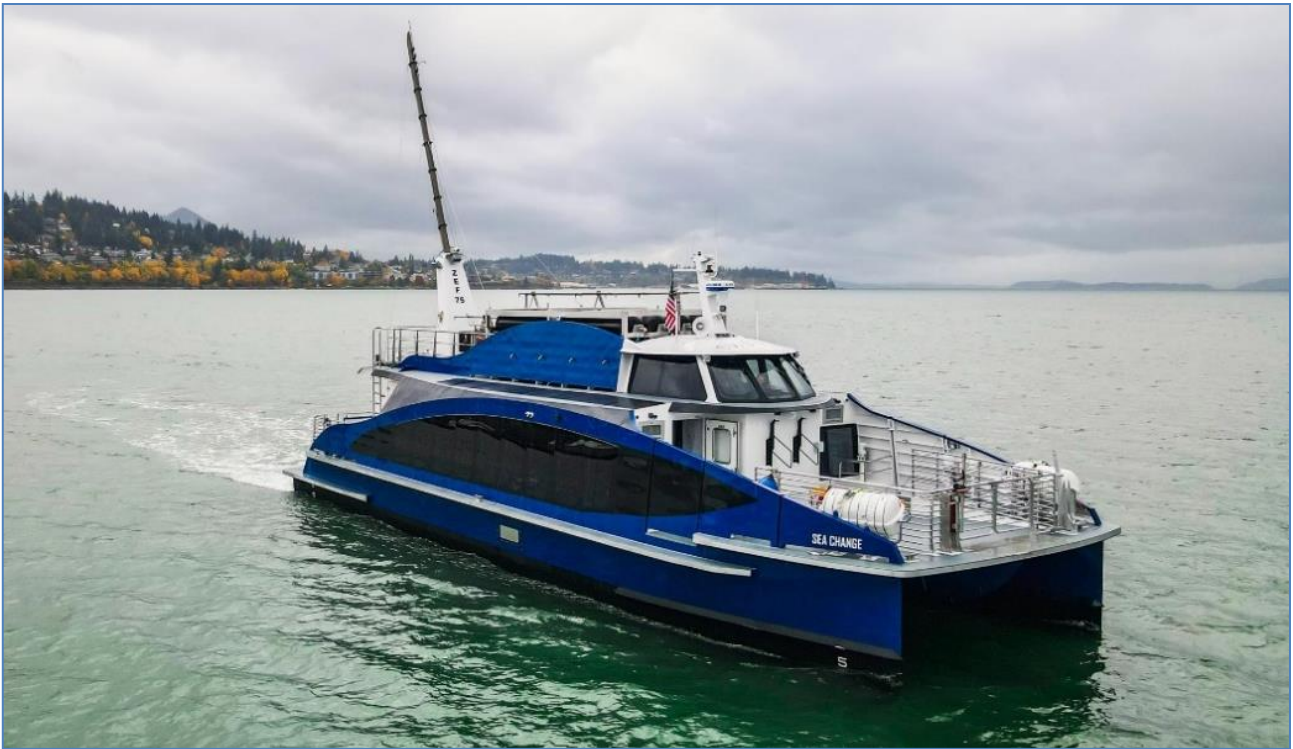
Figure 1 HFC propelled ship „Sea Change“ with an access point in the bow section
