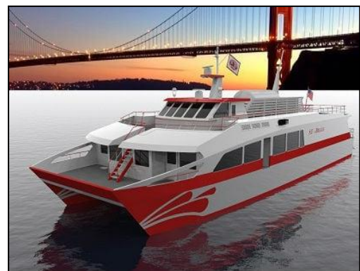
Figure 2 Project of HFC-propelled ship „SF-Breeze“ with access point in mid-section
