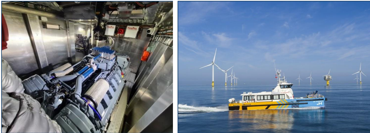
Figure 5 Hydrogen engine onboard powered windcat workboat by MAN (photo: mantruckandbus.com)
